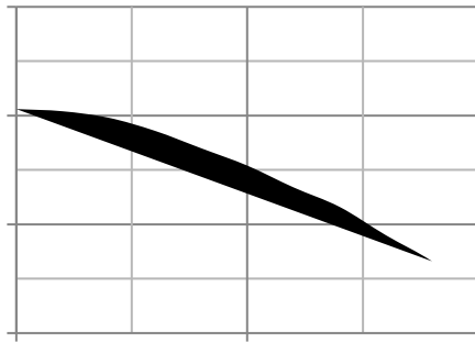
Fig.3 Threshold Voltage V.S Junction Temperature
