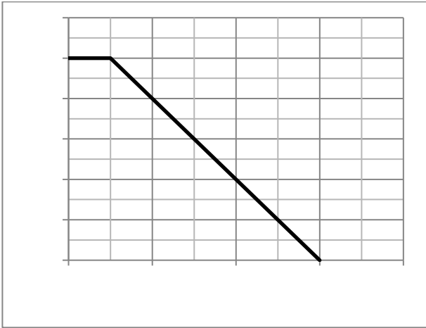
Fig.3 Threshold Voltage V.S Junction Temperature
